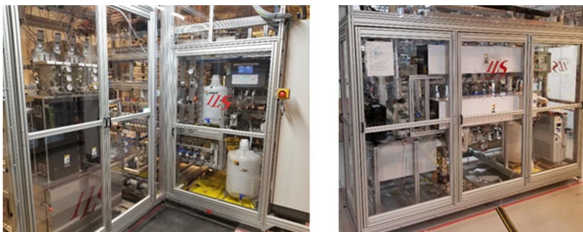
Figure 7: 16 reactors powder Test unit (left) & two cores test unit (right) at Shell Technology Center - Houston.
